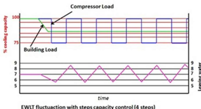
Units with stepless regulation offer benefits that the units with step regulation are unable to match. The ability to follow the system energy demand at any time and the possibility to provide steady outlet water temperature without deviations from the set-point, are the two points that allow you to understand how the optimum operating conditions of a system can be met through the use of a unit with stepless regulation.
